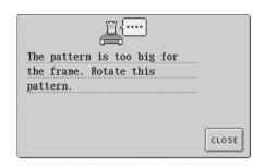
Even after being rotated 90 degrees, embroidery data larger than 200 mm (H)  $\times$  300 mm (W) (approx. 7-7/8 inches (H)  $\times$  11-3/4 inches (W)) cannot be used. (All designs must be within the 200mm(H)  $\times$  300mm(W) (approx. 7-7/8 inches (H)  $\times$  11-3/4 inches (W)) design field size.) For more details, refer to page 113.
